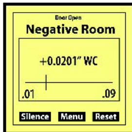
If pressure is Normal, and Door is open, the screen is Yellow
